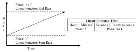
The Linear Flow Rate function is specified by using two Linear Functions Line in two consecutive Program Phases, defined by four parameters:
