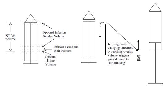
The continuous pumping mode eliminates the problem of flow rate drop-off that is typical with continuous syringe pump systems where one pump is refilling the syringe while the other infuses, and then they switch directions.
